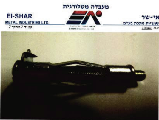
Pic. 7: The Dibble flare is open as flower on tighten up.
