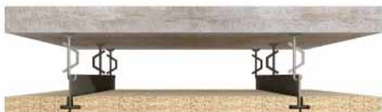
Suspended false ceiling chamfered edges panels mounted on foldaway profiles
