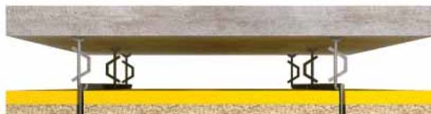
Suspended false ceiling panels mounted on T-shaped profiles, on top of which a thin mineral wool mattress is placed
