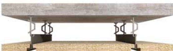
Suspended false ceiling lowered edges panels mounted on T-shaped profiles
