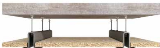
Panels mounted on omega-shaped metal profiles
