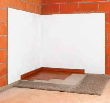
Figure 7 Insulation from floor noises. A continuous layer of Celenit N panels placed between the floor structure and the floor interrupts both noises transmitted through the floor and overhead noises transmitted through the partition wall.
