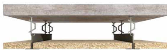
Panels mounted on T-shaped profiles
